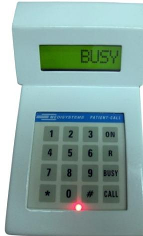
The Desk Unit is a numerical keypad on which the Doctor punches the Case / Call No. of the next patient to be called. Entering this number automatically erases the previous patient's entry. Once the patient enters the room, the Doctor can press the hash key to indicate at the door display that the room is now busy.
