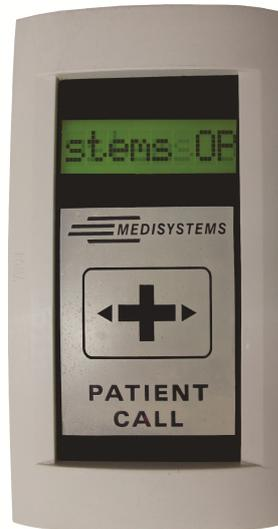
The Door Display Unit is mounted at the room entrance at a height where the calling number is clearly visible. This assists the patient in knowing that he/she is entering the correct room. When the room is occupied this display can also indicate BUSY so that uncalled visitors may not enter and the Doctor has complete privacy with the the patient who is already inside for examination.
